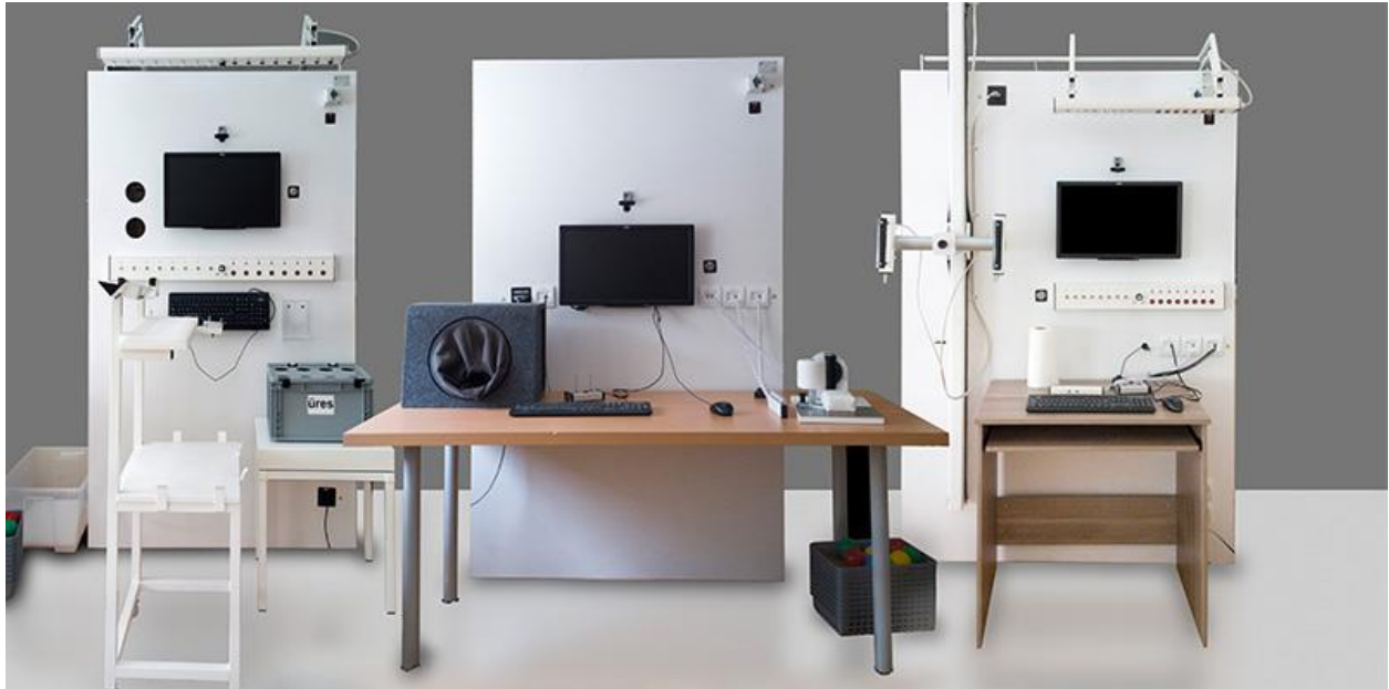
Figure 5. Three measuring panels of ErgoScope work simulator
